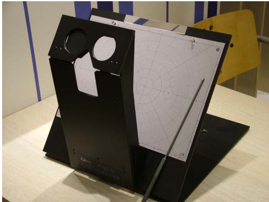
Figure 15: Indigo Visual Field Screener (used to chart motion and colour visual fields) (Heinrich, 2004)
