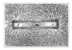
The magnetic behavior of a material depends on its structure (particularly its electron *configuration*), and also on the temperature (at high temperatures, random thermal motion makes it more difficult for the electrons to maintain alignment).
